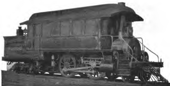
Fig. 31. Four-Coupled Double Ender (2-4-6) Inspection Locomotive. Built by the American Locomotive Co. for the Adirondack & St. Lawrence. Cylinders 16 in. x 22 in., Working Steam Pressure 160 lbs. per sq. in., Diameter of Drivers 60 in., Weight on Drivers 57,000 lbs., Total Weight 134,000 lbs.
